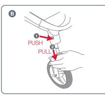
**B** To remove the front wheels, push the release button on wheel moulding.
