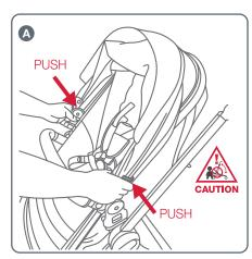
A Place the canopy on the stroller seat and push the clips on the sides of the canopy onto the stroller seat until they snap into place.
