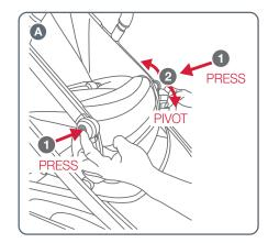
A Press the two release buttons on both sides of the leg rest hinge and hold while raising or lowering the leg rest to the desired position.
