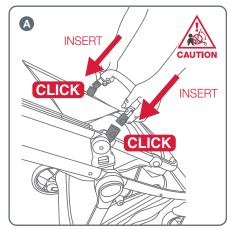
A Insert the arm bar mouldings into the sockets on each side of the stroller frame and push down on the arm bar until you hear a 'click'.
