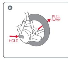
**B** To remove the rear wheels, press and hold the release button in the wheel housing and pull away.
