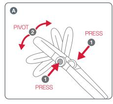
A Press the two release buttons on the outside of the handle and hold while raising or lowering the handle to the desired position.
