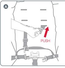
**A** To change the shoulder harness height, push the shoulder harness tongue out of the current harness slot and through the back of the seat.
