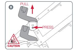
**B** To remove the adaptors, press in and hold the button on the bottom of the adaptor and pull up the adaptors out of the frame sockets.
