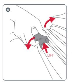
**A** Lift the recline lever on the back of the seat and hold while raising or lowering the backrest to the desired position.
