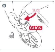
**B** To allow the wheels to swivel, slide the black swivel wheel locking clip towards the outside of the frame until you hear a 'click'.
