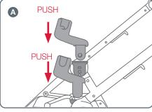
A Engage the stroller brake first. Align the baby capsule adaptors to the stroller frame socket and push down until you hear a 'click' sound and locks into position. Ensure adaptors are locked correctly by pulling up to check.
