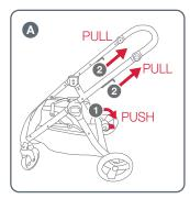
A Engage the brake. Pull the latches on the handle tube upwards and drop down the handle all the way.
