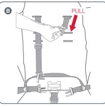
**B** Select the appropriate shoulder harness height and pull each shoulder harness tongue through the harness slot.
