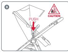
**B** Turn the seat facing opposite direction and then attach the stroller seat to the frame in the rearward facing position.
