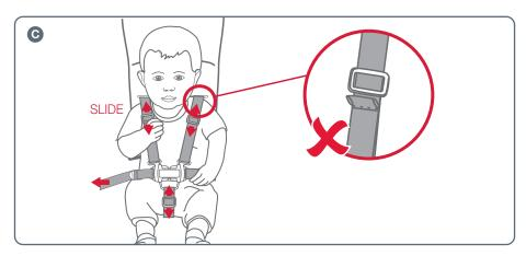
**C** To tighten or loosen the shoulder straps, slide the 3 bar slider up or down to adjust to the desired fit. Always adjust the harness strap when changing the seating position of the child.
