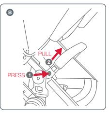
**B** To remove the arm bar, press the button on each side of the arm bar moulding and pull arm bar up and out of the sockets.
