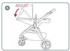
**B** Using the recline lever adjust the backrest to the lowest position.
