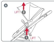
A Lift both release levers on the seat connectors at the same time and lift the seat up and away from the stroller frame.
