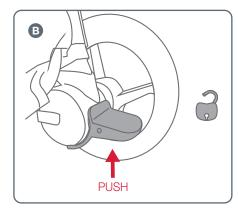
**B** Push the brake pedal upward until the brake is disengaged.
