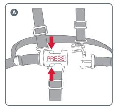
**A** To release the buckle, squeeze the top and bottom buckle tongues together with enough pressure so the buckle tongues can release from the buckle housing.
