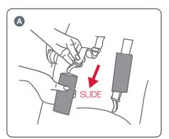
**A** Slide the shoulder harness pads onto the shoulder harness straps and adjust to the position which fits comfortably on the child.
