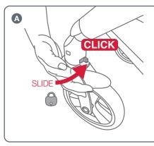
**A** To lock the front wheels into the fixed position, slide the swivel wheel locking clip towards the inside of the frame until you hear a 'click'.
