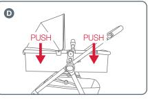
**D** Push down the backrest and leg rest to complete the converting. Use the harness to secure the baby in lay flat mode.
