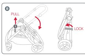
**B** Pull the folding handle under the stroller seat upwards until you hear a 'click' and the frame is fully folded and the frame lock latch is locked in properly.
