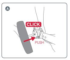
A Insert wheel axle into the moulding and push in until you hear a 'click'. Pull on each wheel to make sure it is securely attached. Repeat the process if not locked in.
