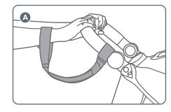
**A** A wrist tether strap is provided hand through the tether strap loop whenever you use the stroller. Only remove your hand from the tether strap loop when the brakes have been applied to the stroller wheels.
