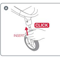
A Insert each front swivel wheel assembly into the wheel moulding and push in until you hear a 'click'. Pull on each wheel to make sure it is securely attached. Repeat the process if not locked in.
