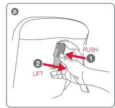
B To lower the backrest, push the button and pull the lever then slowly lower the backrest.
