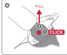
**B** Pull up on the arm bar to ensure it has fully locked in.
