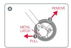
**B** To remove the wheels, pull the metal latch downwards on the underneath of the rear wheel moulding to release the wheel, and then pull the wheel off.
