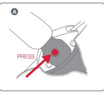
**A** To remove the arm bar, push the red quick release tabs in on the inside of each
