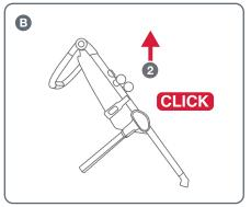
**B** Open the frame as shown by the arrows (2) until you hear a 'click' which indicates the frame is fully opened and locked. Push down on the stroller handle to confirm that the frame is locked.
