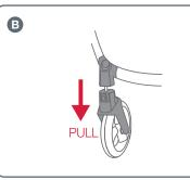
**B** To remove each front swivel wheel, press the grey quick release button on the top of the front leg mouldings
