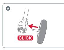
A Insert each wheel axle into the moulding and push in until locked. You should hear a 'click' which indicates the wheel has locked in. Pull on the wheel to make sure it is engaged. Repeat the process if not locked in.
