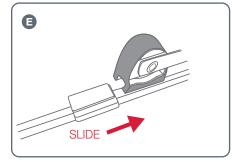
**E** To remove the canopy, slide the canopy mouldings (as shown by the arrow) out of the frame mouldings.
