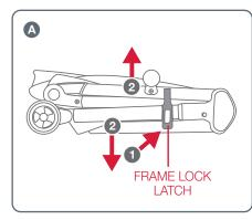
**A** Release the frame lock latch (1) located on the rear leg.
