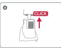
A To attach each front swivel wheel, insert the swivel wheel and push it into the wheel moulding until you hear a 'click' which indicates the wheel is locked in. Pull on each wheel to make sure it is engaged. Repeat the process if not locked in.
