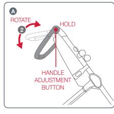
**A** To adjust the handle height, squeeze in and hold the buttons on the outside of the handle. Rotate the handle up or down to the desired position then release the buttons.
