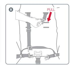
A The stroller seat has 3 sets of harness slots at different heights to accommodate the child. To change the shoulder harness height, push the shoulder harness tongue out of the current harness slot and through the back of the seat fabric. **B** To reposition the harness, pull the shoulder harness buckle tongue through the desired slot.
