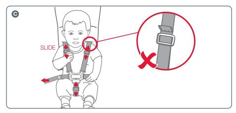
**C** To tighten or loosen the shoulder straps, slide the 3 bar slider up or down to adjust to the desired fit. Always adjust the harness strap when changing the seating position of the child.
