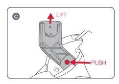
**C** To remove the adaptors, push the button in and pull the adaptors out of the stroller frame sockets.
