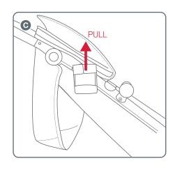
**C** Pull the Cup holder up to remove the Cup holder.
