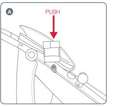
**A** Align the Cup holder with pin on the frame and push down. The Cup holder can only fit on the right hand side of the frame.
