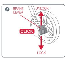
A The red brake lever is located on the right hand side of the stroller beside the rear wheel.
