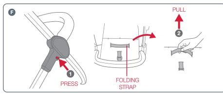
F (1) Press folding button located on the right-hand side of the stroller frame.
