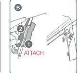
**B** Attach the hook strip (1) on the outside edge of the canopy to the loop strip (2) on the inside edge of the stroller seat side panel.
