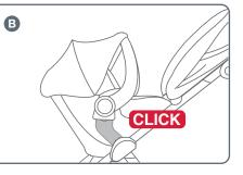
**B** Press down firmly until you hear a 'click' which indicates the baby capsule has locked into position.
