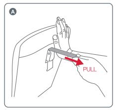
A To raise the backrest, support the backrest with one hand and pull the strap until designed position.
