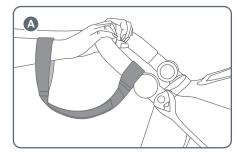
**A** A wrist tether strap is provided, place hand through the tether strap loop whenever you use the stroller. Only remove your hand from the tether strap loop when the brakes have been applied to the stroller wheels.
