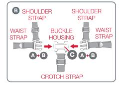
**B** Push both buckle tongues (A + B) into the buckle housing (C) until the buckle tongues lock into position.
