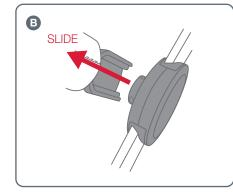
B Slide the arm bar out of the stroller.
