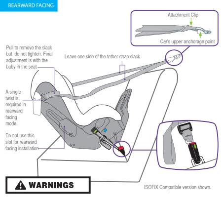
DO NOT USE RESTRAINT IN REARWARD FACING MODE WITHOUT STABILISING BAR FULLY DEPLOYED AND LOCKED THE TOP TETHER STRAP MUST ALWAYS BE FITTED WHEN THE CHILD RESTRAINT IS USED IN A VEHICLE.
