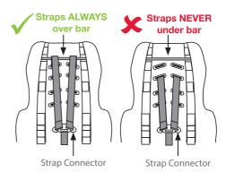
Shoulderstraps must be threaded through appropriate shoulder strap slots then over the top of bar at rear of restraint.
