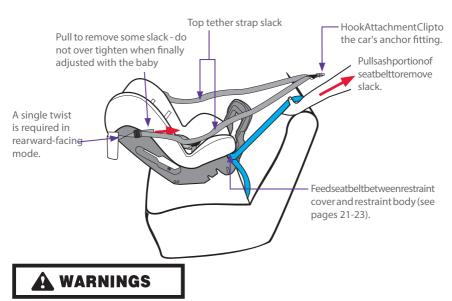
DO NOT USE RESTRAINT IN REARWARD FACING MODE WITHOUT STABILISING BAR FULLY EXTENDED.
