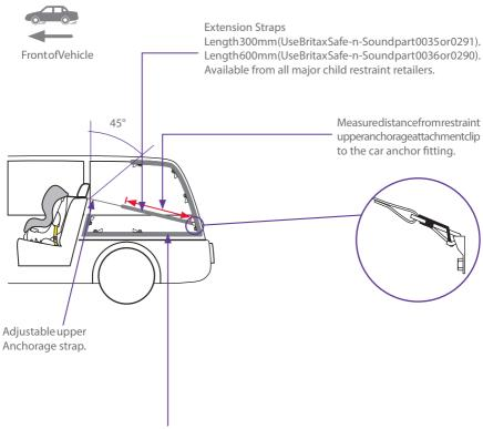
The shaded areas of this diagram illustrate the possible locations of the anchor fitting. With in each shaded area is an anchor fitting showing the correct way to install the fitting. Ensure the anchor fitting is aligned as illustrated unless stated otherwise in the vehicle owner's handbook.
