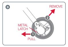
**B** To remove the wheels, pull the metal latch downwards on the underneath of the rear wheel moulding to release the wheel, and then pull the wheel off.
