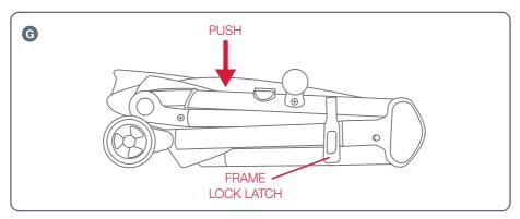
**G** Lock the frame with the frame lock latch located on the right hand side of the stroller, push stroller down until the frame lock is engaged. Ensure frame is securely locked.
