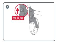
A To lock the swivel wheels, push the swivel lock up on the front of each wheel until you hear a 'click'.
