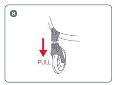
**B** To remove each front swivel wheel, press the grey quick release button on the top of the front lea mouldings
