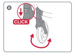
**B** To allow the wheels to swivel, push the swivel lock down on the front of each wheel until you hear a 'click'.
