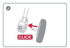
A Insert each wheel axle into the moulding and push in until locked. You should hear a 'click' which indicates the wheel has locked in. Pull on the wheel to make sure it is engaged. Repeat the process if not lockedin.
