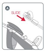
A To attach the canopy, slide the canopy mouldings (as shown by the arrow into the frame mouldings until they lock together.
