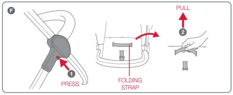
F Press the folding button (1) located on the right hand side of the stroller. With the other hand pull up on the folding strap (2) located on the seat (as shown by the arrow). The stroller will begin to fold as you pull the strap up, continue to fold until the frame lock is engaged.
