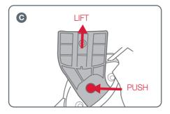
C To remove the Click & Go<sup>™</sup> adaptors, press the button and pull up the adaptors out of the frame sockets.
