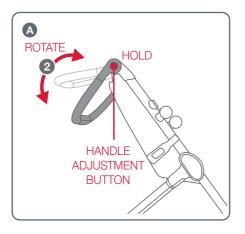
A To adjust the handle height, squeeze in and hold the buttons on the outside of the handle. Rotate the handle up or down to the desired position then release the buttons.
