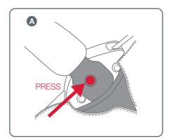
A To remove the arm bar, push the red quick release tabs in on the inside of each stroller hinge.
