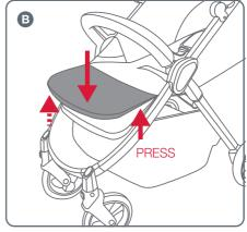
**B** To lower the leg rest, press the lever under the leg rest on both sides and lower the leg rest.
