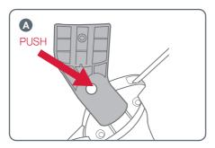
A Align the Click & Go™ adaptors to stroller frame sockets and push down.
