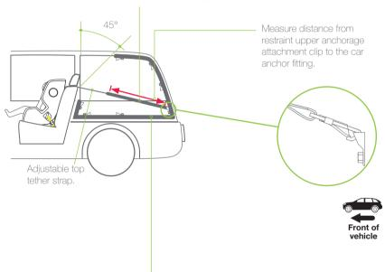
The shaded areas of this diagram illustrate the possible locations of the upper anchorage point (car anchor fitting). Within each shaded area is an upper anchorage point showing the correct way to install the fitting. Ensure the upper anchorage point is aligned as illustrated unless stated otherwise in the vehicle owner's handbook.
