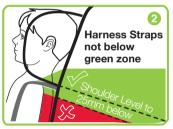
Step 2. Adjust headrest height to suit child. The shoulder straps must be in the slots which are nearest to the child's shoulders, but not more than 25mm below the child's shoulders.
