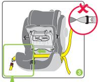
Step 3. Lengthen vehicle seatbelt. Feed vehicle seatbelt through yellow FORWARD FACING BELT PATH guide. across the seat and through opposite belt auide.
