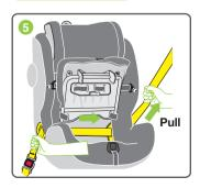
Step 5. Remove any slack from the vehicle seatbelt by pulling the webbing through the buckle, and back towards the sash-belt.
