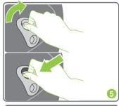
Step 5. To open CLICKTIGHT™ frame, twist and push the CLICKTIGHT™ button. Lift frame.
