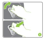
Step 1. To open CLICKTIGHT™ frame, twist and push the CLICKTIGHT™ button. Allow frame to lift.
