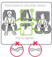
Step 3. Fit the shoulder straps over the child's shoulders ensuring they do not become twisted. Engage both tongues into the buckle.
