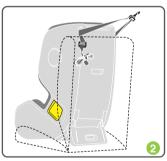
Step 2. Ensure child seat is against vehicle seatback and top tether is not trapped behind seat.
