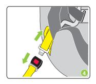
Step 4. Disengage the vehicle seatbelt buckle.
