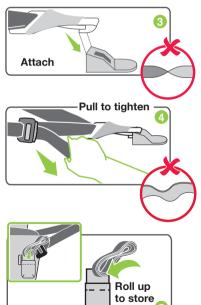
Step 3. Connect top tether attachment clip to vehicle anchor fitting.
