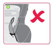
Step 6. Ensure no part of the harness assembly is trapped under the CLICKTIGHT™ frame before closing.
