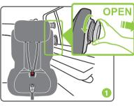
Step 1. Rotate the SICT<sup>TM</sup> anti clockwise to full extension on the preferred door side for both the torso and headrest.
