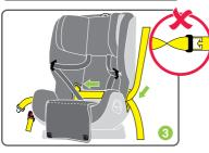
Step 3. Feed vehicle seatbelt through yellow FORWARD FACING BELT PATH guide, across the seat and out the opposite guide.
