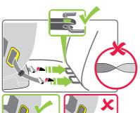
Step 7. Connect ISOFLEX® connectors to ISOFIX low anchorages on each side. See vehicle manual to locate ISOFIX
