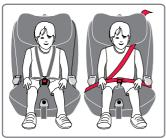
A convertible booster seat with in-built harness until approximately 4 years old and then as a booster seat with vehicle lap-sash seatbelt until approx 6 to 8 years of age (or seatbelt and compatible child harness).
