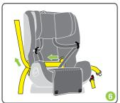
Step 6. Remove vehicle seatbelt from yellow Forward Facing Belt Path. Replace middle cover.
