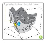
Step 6. Temporarily place top tether and attachment clip over the back of child seat.
