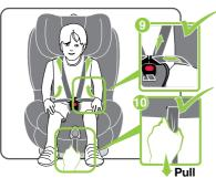
Step 9. Remove all slack from the lap strap area (including behind child's bottom), by pulling up on the shoulder straps.
