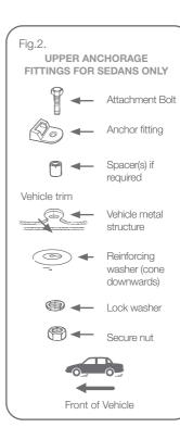
ONLY USE A 5/16 UNC GRADE 5 BOLT. IF THE BOLT IS NOT THE CORRECT LENGTH THE CAR MANUFACTURER'S HAND BOOK CAN PROVIDE ADVICE ON THE CORRECT LENGTH BOLT.
