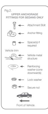
ONLY USE A 5/16 UNC GRADE 5 BOLT, IF THE BOLT IS NOT THE CORRECT LENGTH THE CAR. MANUFACTURER'S HAND BOOK CAN PROVIDE ADVICE ON THE CORRECT LENGTH BOLT.
