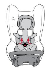
F. Fit either harness tongue into the harness buckle followed by the other tongue. A click is heard when the last tongue is fully engaged. Should the second tongue not engage - press the red button and reinsert the tongues. Ensure secure engagement by pulling harness straps. If the harness buckle does not engage correctly then it may require cleaning or seek replacement - refer to page 55. The buckle tongues are fully engaged when both tongues are inserted and a 'click' is heard.
