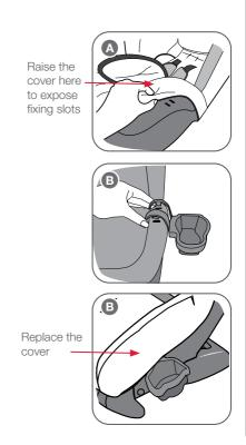
Consult the vehicle owner's handbook for location of anchorage fittings or anchorage points and the possible use of spacers. Some vehicles may have an anchor fitting fitted by the vehicle manufacturer. If anchorage points cannot be found refer to car manufacturer or local child restraint fitting station or traffic authority for optimum position of anchorage point and the use of spacers.
