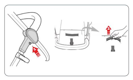
G Lock the frame with the frame lock latch.
