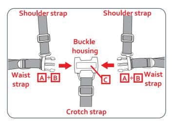
**C** Push both buckle tongues (**A** + **B**) into the buckle housing (**C**) until the buckle tongues lock into position.
