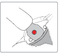
**B** To remove the arm bar, push the red quick release tabs in on the inside of each stroller hinge and slide the arm bar out of the stroller.
