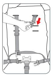
I To reposition the harness, pull the shoulder harness buckle tongue through the desired slot.
