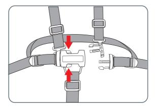
**G** To release the buckle, squeeze the top and buckle tongues together with enough pressure so the buckle tongues can release from the buckle housing.
