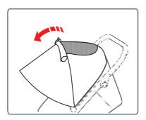
**E** To remove the canopy, slide the canopy mouldings (as shown by the arrow) out of the frame mouldings.
