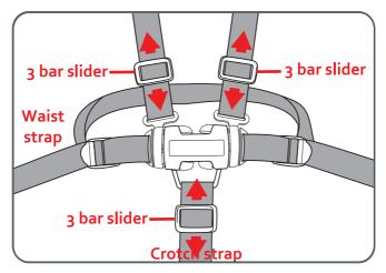
**D** Tighten or loosen crotch straps by sliding the 3 bar sliders up or down.
