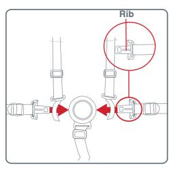
PLEASE NOTE: Each waist buckle tongue has a raised rib on one side and can only be locked into the buckle assembly with the raised rib facing up.
