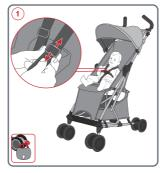
Do not slide 3 bar slider over the sewn tab on the shoulder harness. Adjusting the shoulder harness strap height
