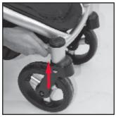
A For swivel wheel mode slide both red latches up until they lock it into position.
