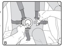
C Tighten or loosen the shoulder straps and crotch strap by sliding the 3 bar harness adjuster up or down.
