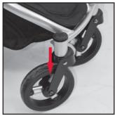
B To lock the front wheels into the fixed position, slide both red latches down until they lock.
