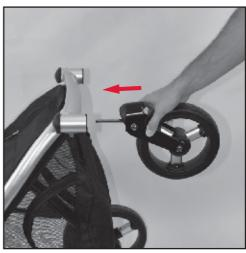
A Take each front wheel assembly and push the axle into the wheel housing, until it locks in.
