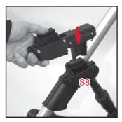
A Align the adaptor with the stroller frame mouldings as the adaptor extends towards the front of the stroller and the ribbed section of the mouldings face inwards
