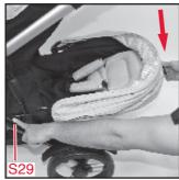
Continue to lower the second seat, the foot end of the second seat will slide up the frame to the folded position.
