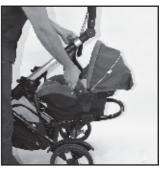
For easier installation, remove stroller seat or infant carrier from frame, (see sections 1.15 (b) & 3.2 (O)). The infant carrier must face towards the front of the stroller. With the infant carrier handle in the upright position, locate the infant carrier handle mouldings on either side, directly over the second seat frame mouldings. Notice the indicator is GREEN.
