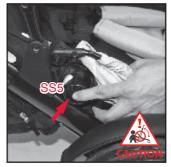
With the second seat in the folded position, locate the release buttons (SS5) on the sides of the second seat frame.
