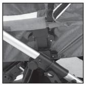
L Line up plastic moulding on sides of bassinet with sockets in the middle of the stroller frame.
