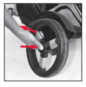
C To release the rear wheels, press in and hold the central button. Then slide the wheel out and remove. Repeat for the other side.
