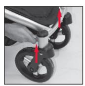
C For swivel wheel mode, lift the swivel latch up on both front wheels until they lock into position.
