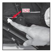
B While still holding the backrest adjusting lever up, press the safety lock button (\$29), and continue to lower the head end of the second seat.
