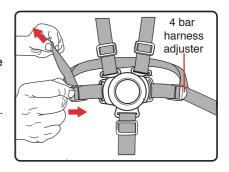
**E** Release the harness by depressing the button in the centre of the buckle while pulling the two waist tongues away from the buckle assembly.
