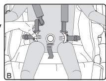
Press in & hold the centre crotch buckle button and insert the waist buckle tongues into the crotch buckle assembly.
