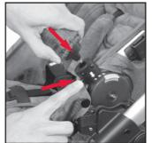
**B** Press in and hold the engaging/release button, then insert the pin all the way in.
