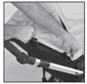
B Attach the canopy hook strips to the pile strips around the top and sides of the frame for a secure fit.
