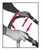
B Press both buttons in together and hold. Now rotate the handle up or down to the desired height position.
