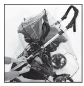
F Join the hook and pile around the handle tube.
