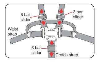
C Tighten or loosen shoulder and crotch straps by sliding up and down the 3 bar sliders.
