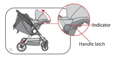
B Continue to rotate the handle forward until it returns to the upright position. Release the latches, the indicator should now be GREEN.
