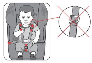
Tighten or loosen the shoulder straps, slide the 3 bar slider up or down to adjust to the desired fit. Always adjust the harness strap when changing the seating position of the child.
