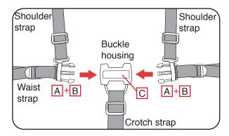
B Push both buckle tongues (A+B) into the buckle housing (C) until the buckle tongues lock into position.
