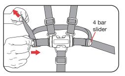
D Tighten or loosen the waist straps, hold and lift the 4 bar slider and then pull the harness strap, to adjust to the desired fit. The waist strap needs to fit firmly around the child.
