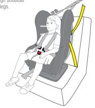
C. Fit either harness tonque into the harness buckle followed by the other tongue until a click is heard. Should the second tongue not insert, press the red button and reinsert the tongues. Ensure secure engagement by pulling the harness straps.
