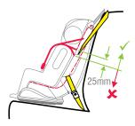
Shoulder straps **must** be threaded through the appropriate shoulder strap slots and then over the top of the bar at the rear of the restraint.
