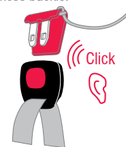
Remove SLIDEGUARD™ converter and engage in harness buckle.
